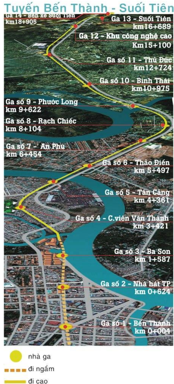
Figure 9 – Ben Thanh-Suoi Tien Metro Line (Line 1) and stations (Source: Management Authority for Urban Railways, 2012)
